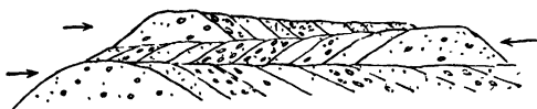
FIG. 46.—Section to show the formation of false-bedding by currents, which are indicated by arrows.
